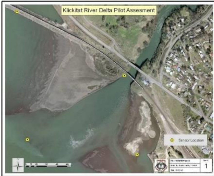
Figure 19. Locations for sensors sampling water temperature, water surface elevation, wind direction, and wind speed for the Klickitat River delta.
