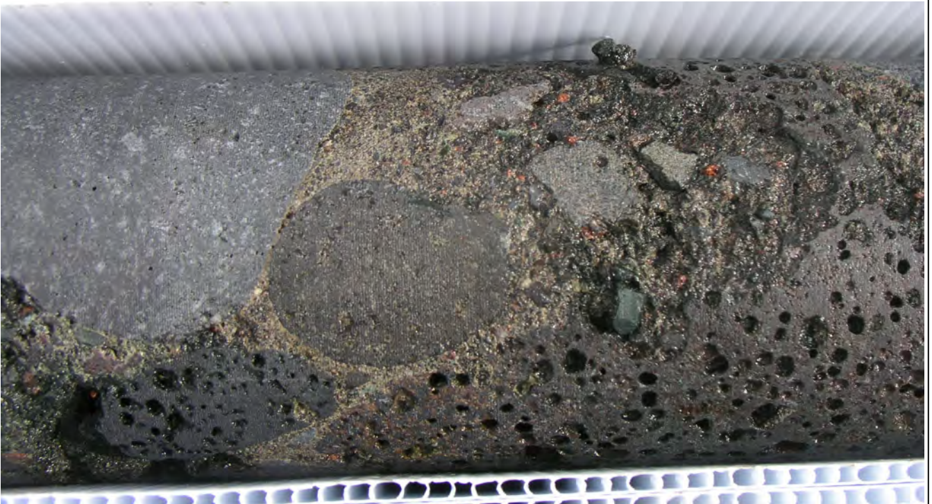
Plate 3b: BH-2 volcanic conglomerate / breccia bedrock.
