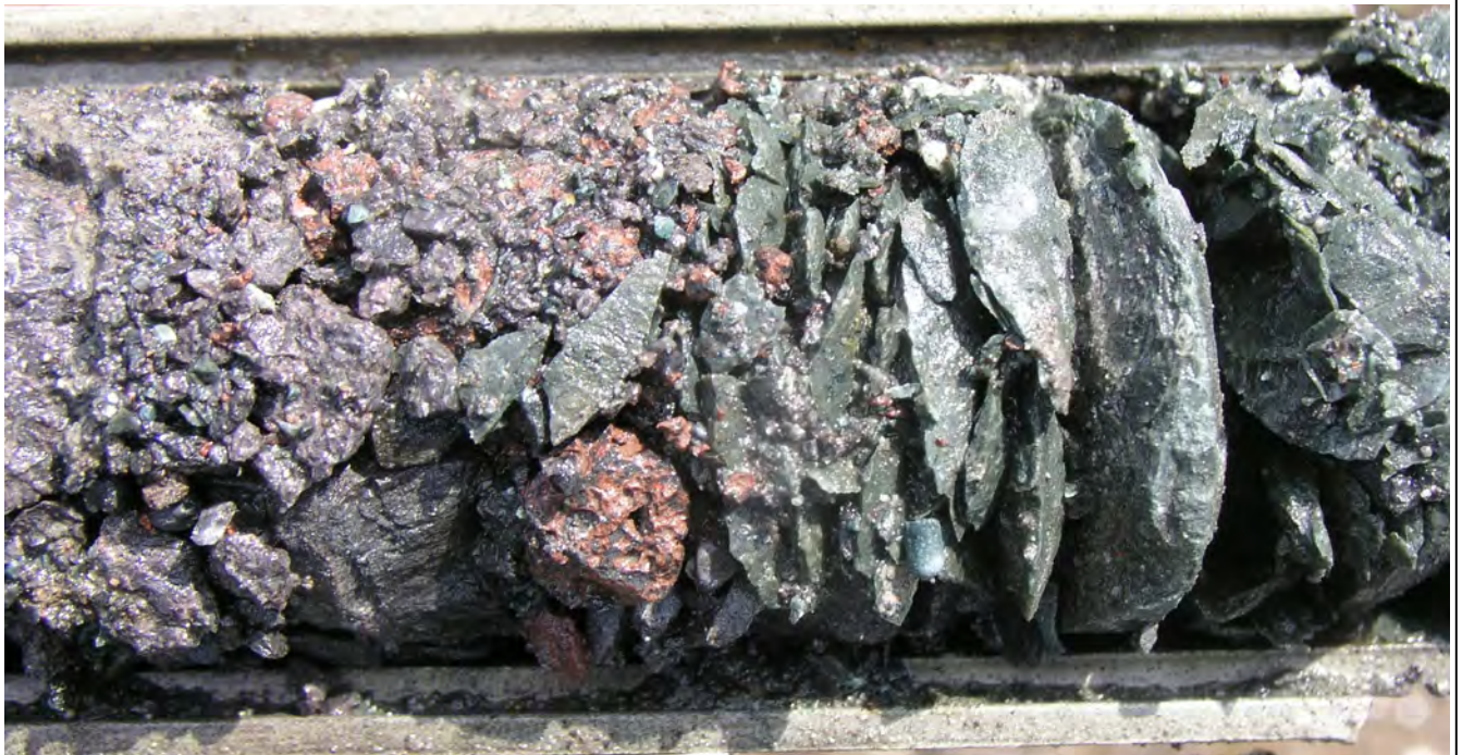
Plate 3a: BH-3 mixed lithology gravel, cobbles and sand.
