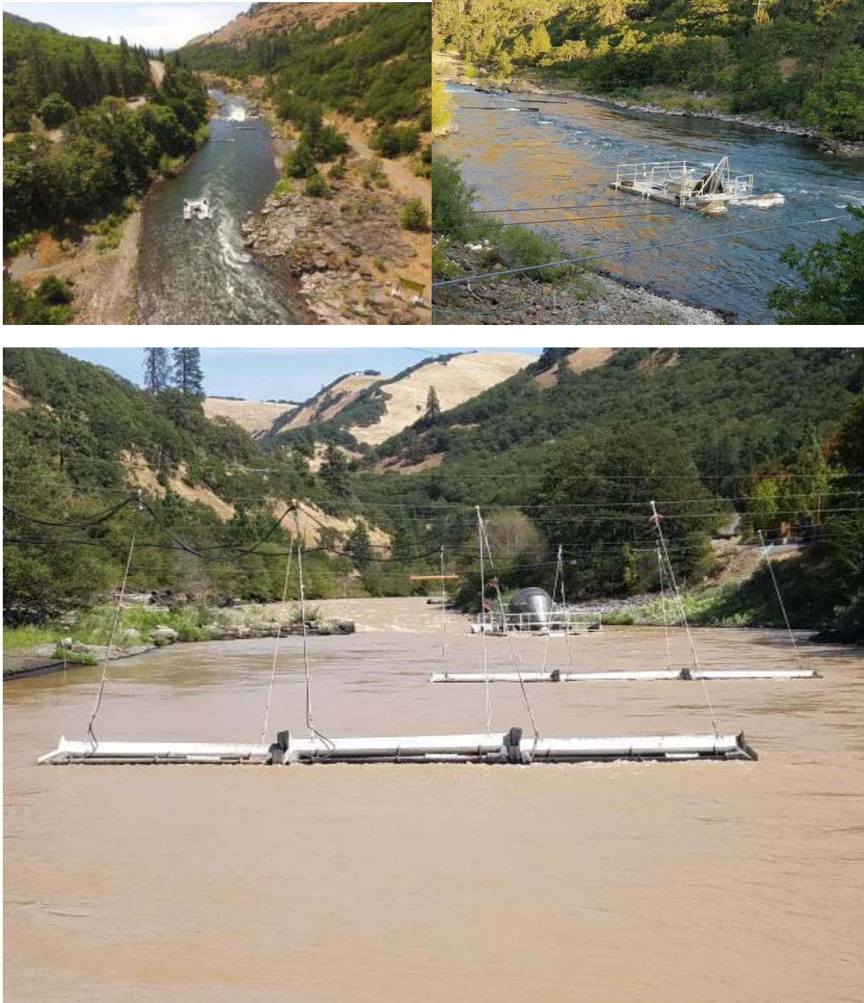
Figure 17. Photos of the rotary screw trap and floating PIT tag interrogation array at river kilometer 4.5. Photo descriptions starting at top left and proceeding clockwise: aerial view looking north to south, downstream view from east bank, and upstream view at the channel level (aerial photos by David Lindley).
